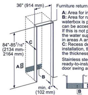
A: Area for installation of power connection.
