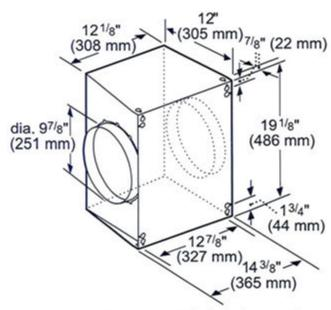
measurements in inches and mm
