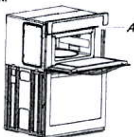
A. Model/serial/rating plate
