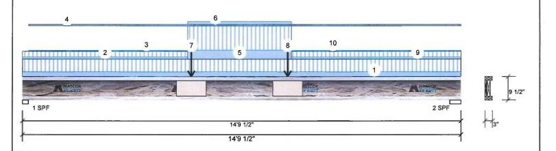
.Continued from page 1 ID Load Type Location Trib Width Side Dead Live Wind Comments Snow 8 Point 8-11-6 Near Face 66 lb 133 lb 0 lb 0 lb 9 9-0-14 to 14-9-8 (Span)0-4-15 Top 15 PSF 40 PSF 0 PSF 0 PSF Tie-In 10 Part. Uniform 9-0-14 to 14-9-8 1 PLF 0 PLF 0 PLF 0 PLF Top
