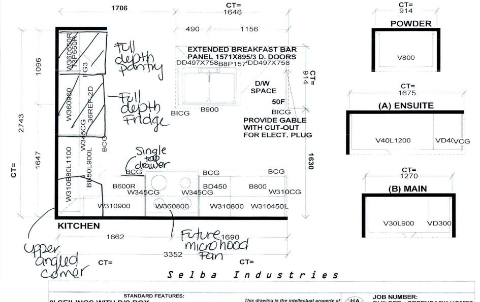
9' CEILINGS WITH D/C BOX 1040MM HIGH UPPER CABINETS DISHWASHER SPACE **DUMMY DOORS ON EXPOSED BACKS** LAMINATE KITCHEN & VANITY COUNTERTOPS This drawing is the intellectual property of SELBA INDUSTRIES INC. and is an original design which must not be released or copied unless applicable fee has been paid or job order placed.
