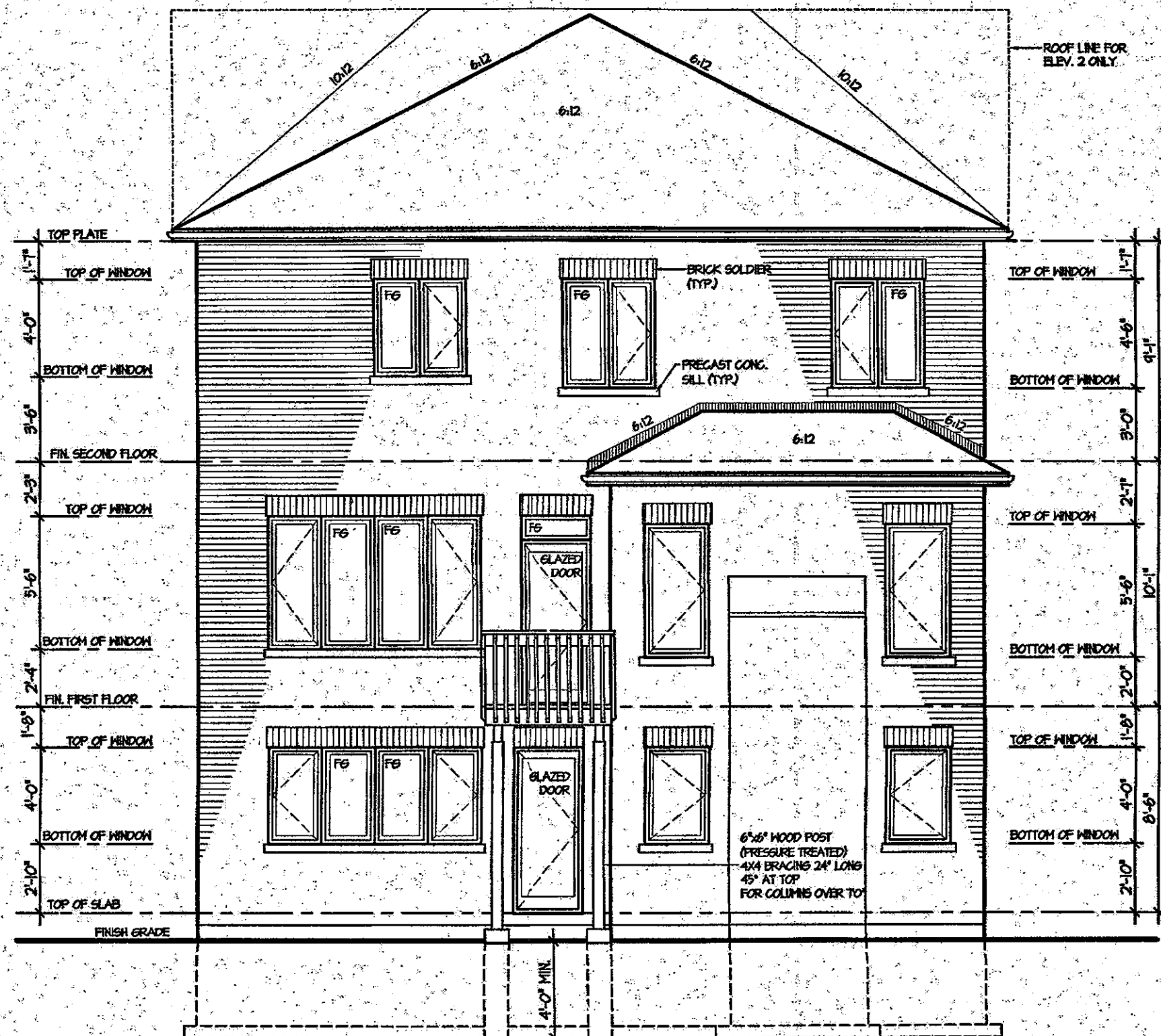
REAR ELEVATION 1, 2 & 3 FOR WALK OUT BASEMENT CONDITION
