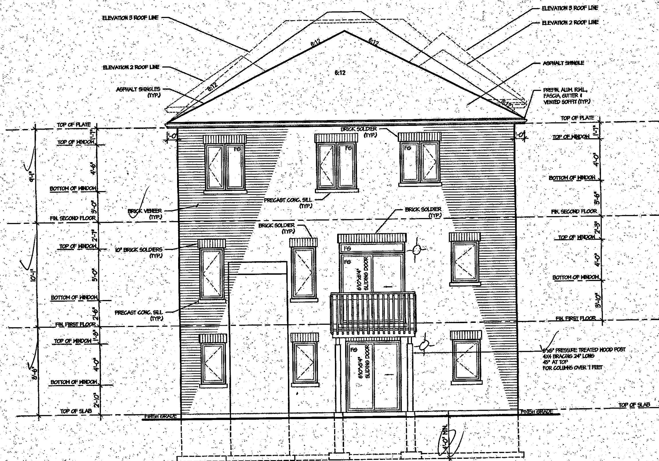
REAR ELEVATION 1, 2 & 3 FOR WALK OUT BASEMENT CONDITION
