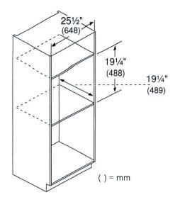
**NOTICE:** The cabinet base must be flat and capable of supporting a weight of at least 142 lbs (64.1 kg).
