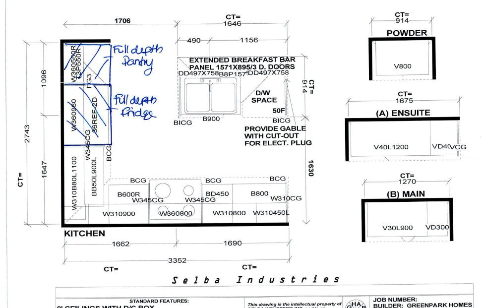
9' CEILINGS WITH D/C BOX 1040MM HIGH UPPER CABINETS DISHWASHER SPACE **DUMMY DOORS ON EXPOSED BACKS** LAMINATE KITCHEN & VANITY COUNTERTOPS This drawing is the intellectual property of SELBA INDUSTRIES INC. and is an original desigh which must not be released original desigh which must not be released to the second unless applicable fee has been paid or job order placed.
