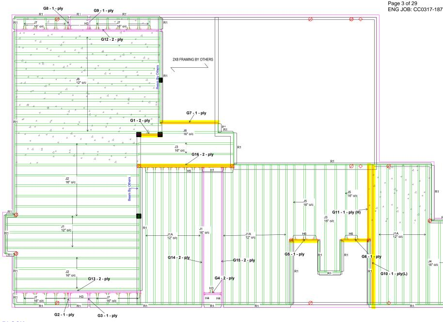
PASS-THRU FRAMING SQUASH BLOCK IS REQUIRED AT ALL POINT LOADS **OVER BEARINGS.**
