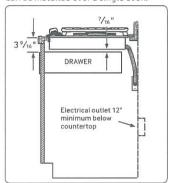
All horizontal clearances must be maintained for a minimum of 18" above the cooking surface
