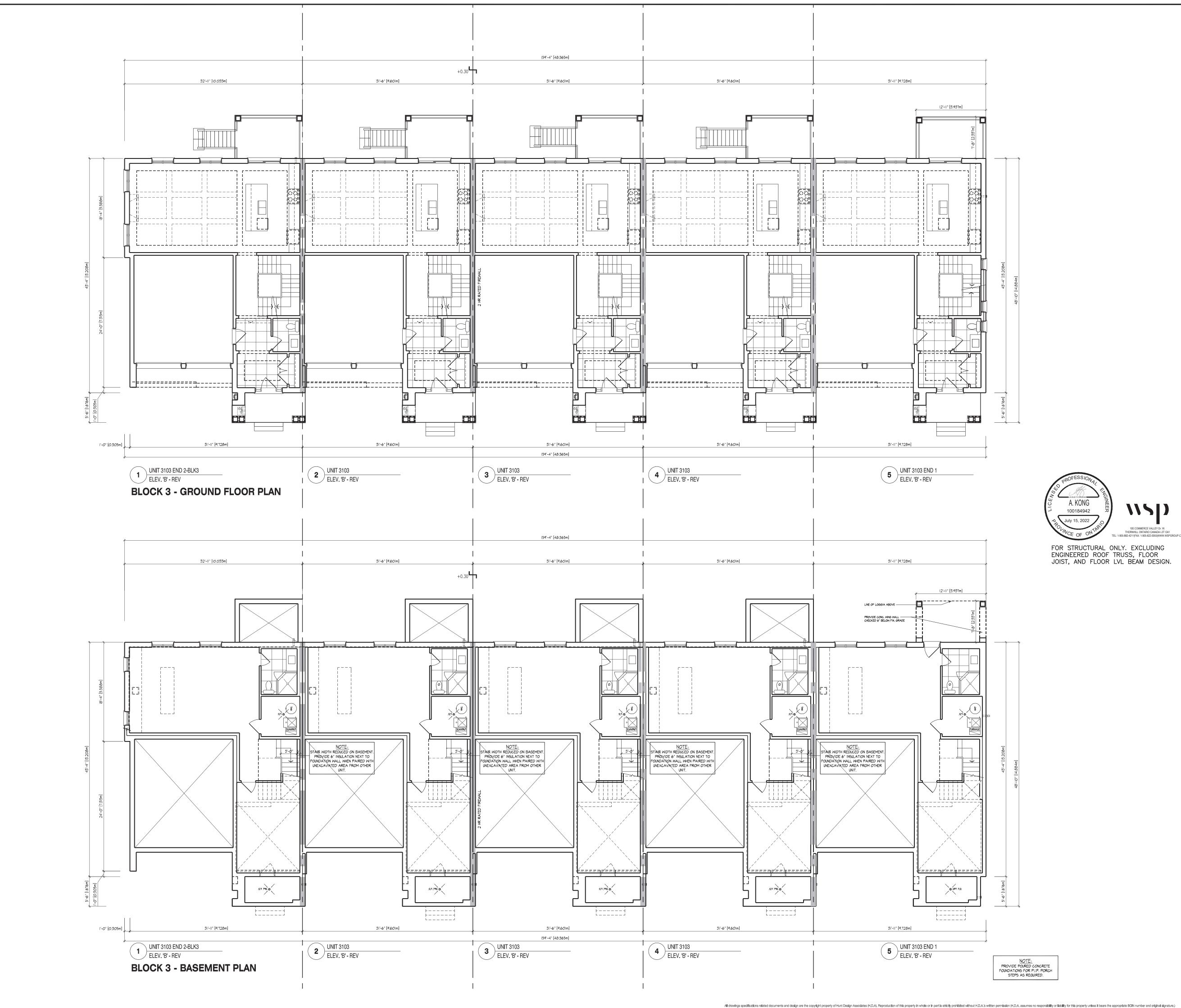
BUILDING AREA 7101.74 sq ft INCLUDING COLD CELLARS 659.77 sq m A FIREWALL IS REQUIRED IF THE BUILDING AREA IS GREATER THAN 600 m2 (6458 sq ft) AS PER BUILDING CODE PART 9 LIMITATIONS SECTION 1.1.2.4.(1) \*\* DEFINITION OF BUILDING AREA AS PER PART 1.4.1.2 IS THE EXTENT OF THE GREATEST HORIZONTAL BUILDING EXTERIOR WALLS ABOVE GRADE TO IF REQ'E THE CENTER OF THE FIREWALL (DEMISING LINE)
