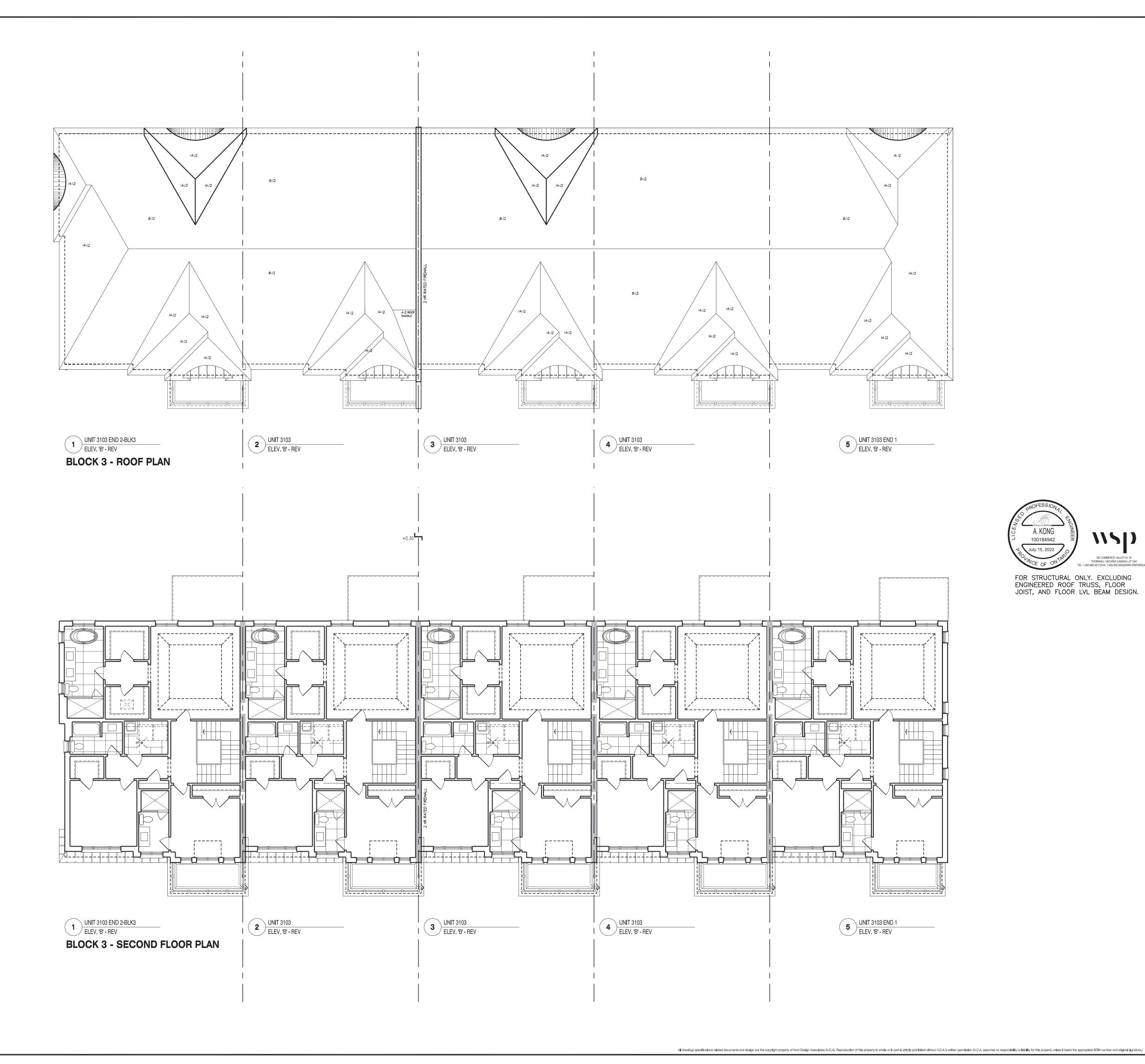
BUILDING AREA 7101.74 sq ft INCLUDING COLD CELLARS 659.77 sq m A FIREWALL IS REQUIRED IF THE BUILDING AREA IS GREATER THAN 600 m2 (6458 sq ft) AS PER BUILDING CODE PART 9 LIMITATIONS SECTION 1.1.2.4.(1) \*\* DEFINITION OF BUILDING AREA AS PER PART 1.4.1.2. IS THE EXTENT OF THE GREATEST HORIZONTAL BUILDING EXTERIOR WALLS ABOVE GRADE TO IF REQ'D THE CENTER OF THE FIREWALL (DEMISING LINE)
