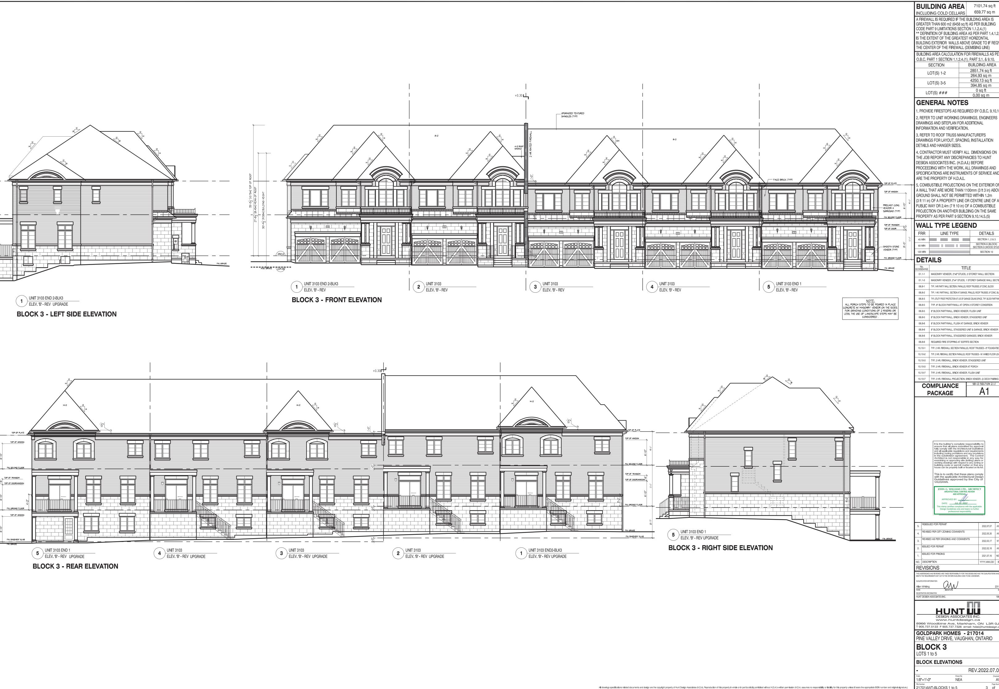
**BUILDING AREA** 7101.74 sq ft 659.77 sq m INCLUDING COLD CELLARS A FIREWALL IS REQUIRED IF THE BUILDING AREA IS GREATER THAN 600 m2 (6458 sq ft) AS PER BUILDING CODE PART 9 LIMITATIONS SECTION 1.1.2.4.(1) \*\* DEFINITION OF BUILDING AREA AS PER PART 1.4.1.2. IS THE EXTENT OF THE GREATEST HORIZONTAL BUILDING EXTERIOR WALLS ABOVE GRADE TO IF REQ'D THE CENTER OF THE FIREWALL (DEMISING LINE) BUILDING AREA CALCULATION FOR FIREWALLS AS PE
