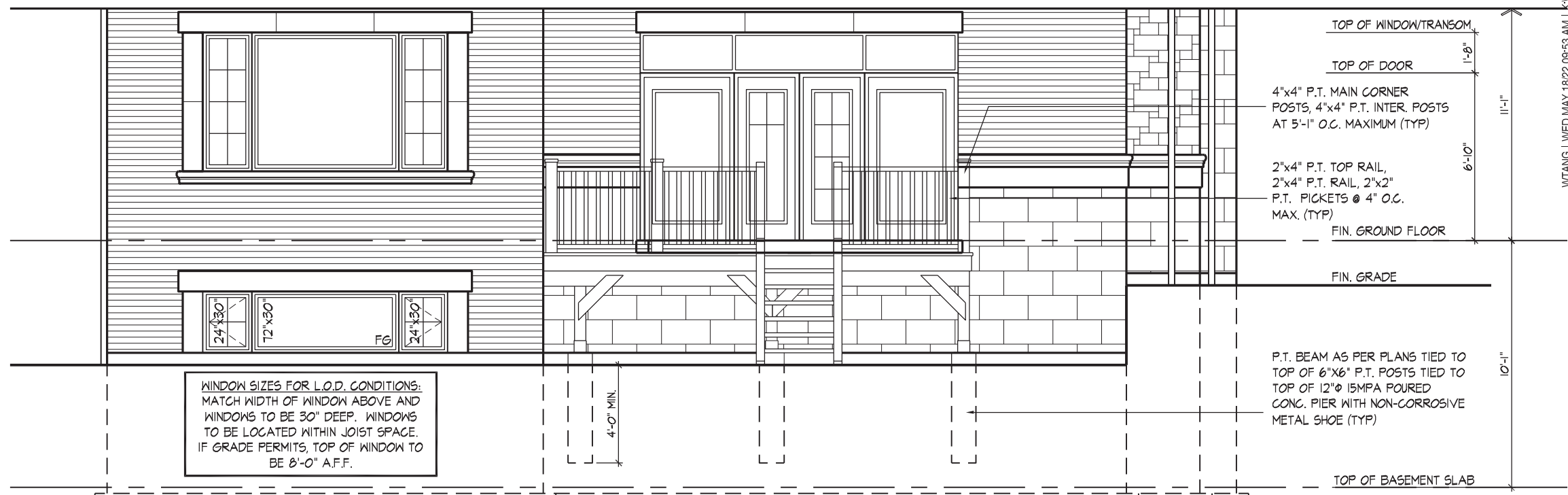
PART. REAR ELEVATION 'A' CORNER - L.O.D. CONDITION
