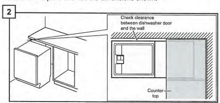
If the dishwasher is to be installed in a corner, ensure that there is adequate clearance to open the door as shown.
