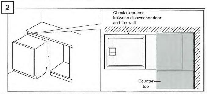
If the dishwasher is to be installed in a corner, ensure that there is adequate clearance to open the door as shown.
