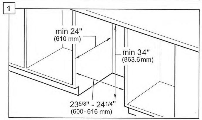
Note: This dishwasher is designed to be enclosed on the top, back and both sides by standard residential kitchen cabinetry.
