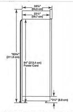
\*When leveling legs are fully extended to 11/4" (3.2 cm) below rollers, add 11/2" (2.9 cm) to the height dimensions.
