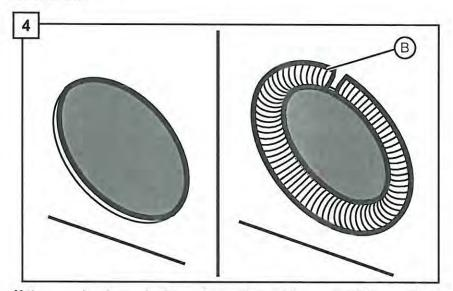
If the opening is made through wood, sand it smooth. If the opening is made through metal, use the provided edge protector (B) or other approved method to protect wiring from damage.
