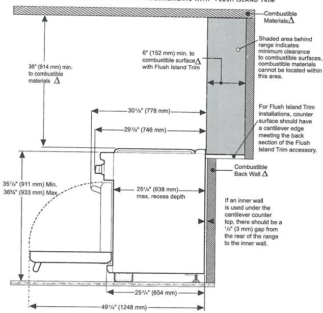
\$\times\$ As defined in the "National Fuel Gas Code" (ANSI Z223.1, Current Edition). Clearances from non-combustible materials are not part of the ANSI Z21.1 scope and are not certified by CSA. Clearances of less than 6" (152 mm) must be approved by the local codes and/or by the local authority having jurisdiction.
