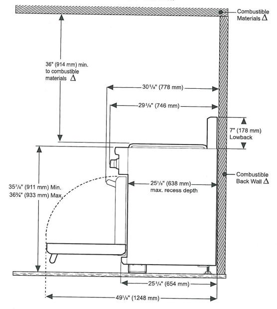
\$\times\$ As defined in the "National Fuel Gas Code" (ANSI Z223.1, Current Edition). Clearances from non-combustible materials are not part of the ANSI Z21.1 scope and are not certified by CSA. Clearances of less than 6" (152 mm) must be approved by the local codes and/or by the local authority having jurisdiction.
