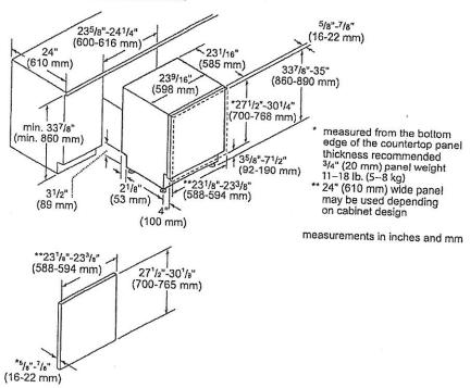
thickness recommended  $^{3}/4"$  (20 mm), panel weight 11–18 lb. (5–8 kg) 24" (610 mm) wide panel may be used depending on cabinet design
