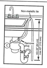
Note: Plumbing installations will vary - refer to local codes. Drain hose included is 79" (201 cm) and can be extended to a maximum of 155 3/4" (396 cm).
