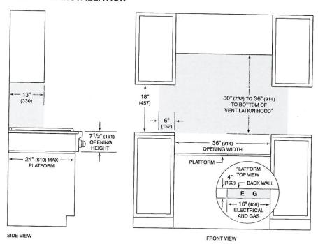
"Without ventilation hood, 36" (914) minimum clearance countertop to combustible materials, 44" (118) for charbroiler. NOTE: Shaded area above countertoy indicates minimum clearance to combustible surfaces, combustible materials cannot be located within this area.
