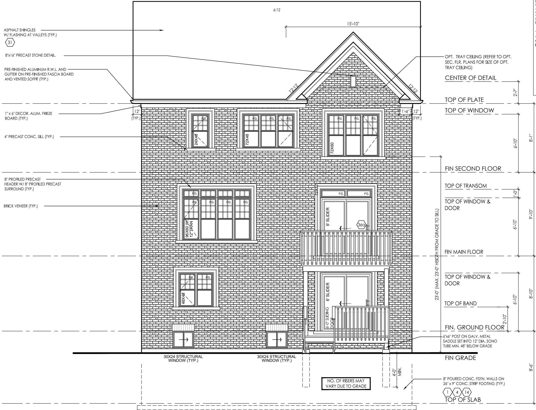
REAR UPGRADE ELEVATION 'B' OPT. GRND / WALK-OUT DECK CONDITION
