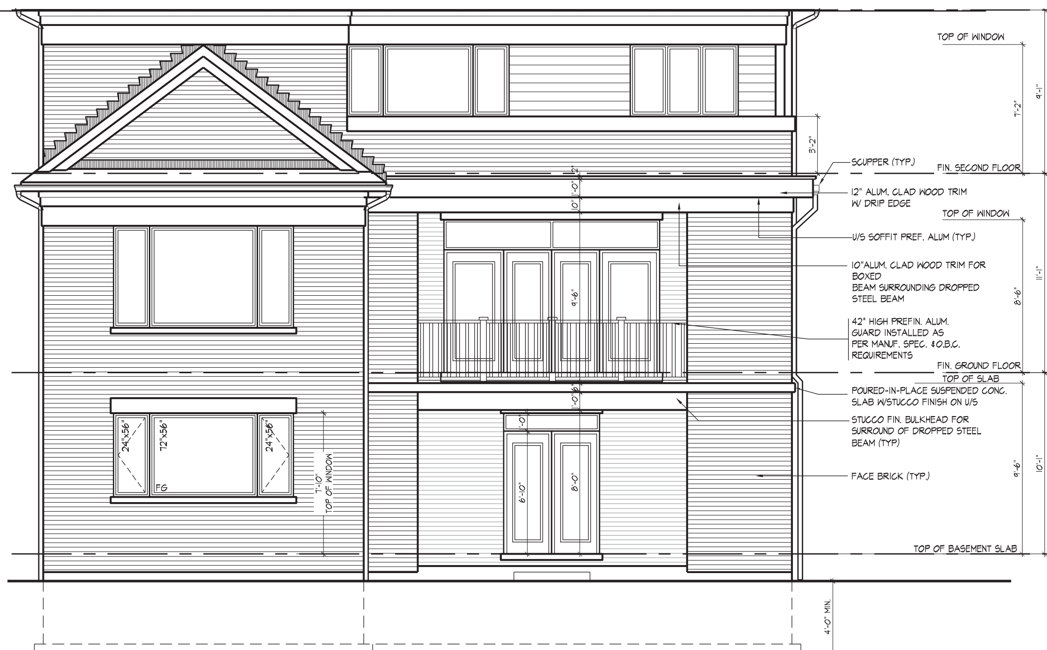
PART. REAR ELEVATION 'C' (LOGGIA/W.O.B. CONDITION)
