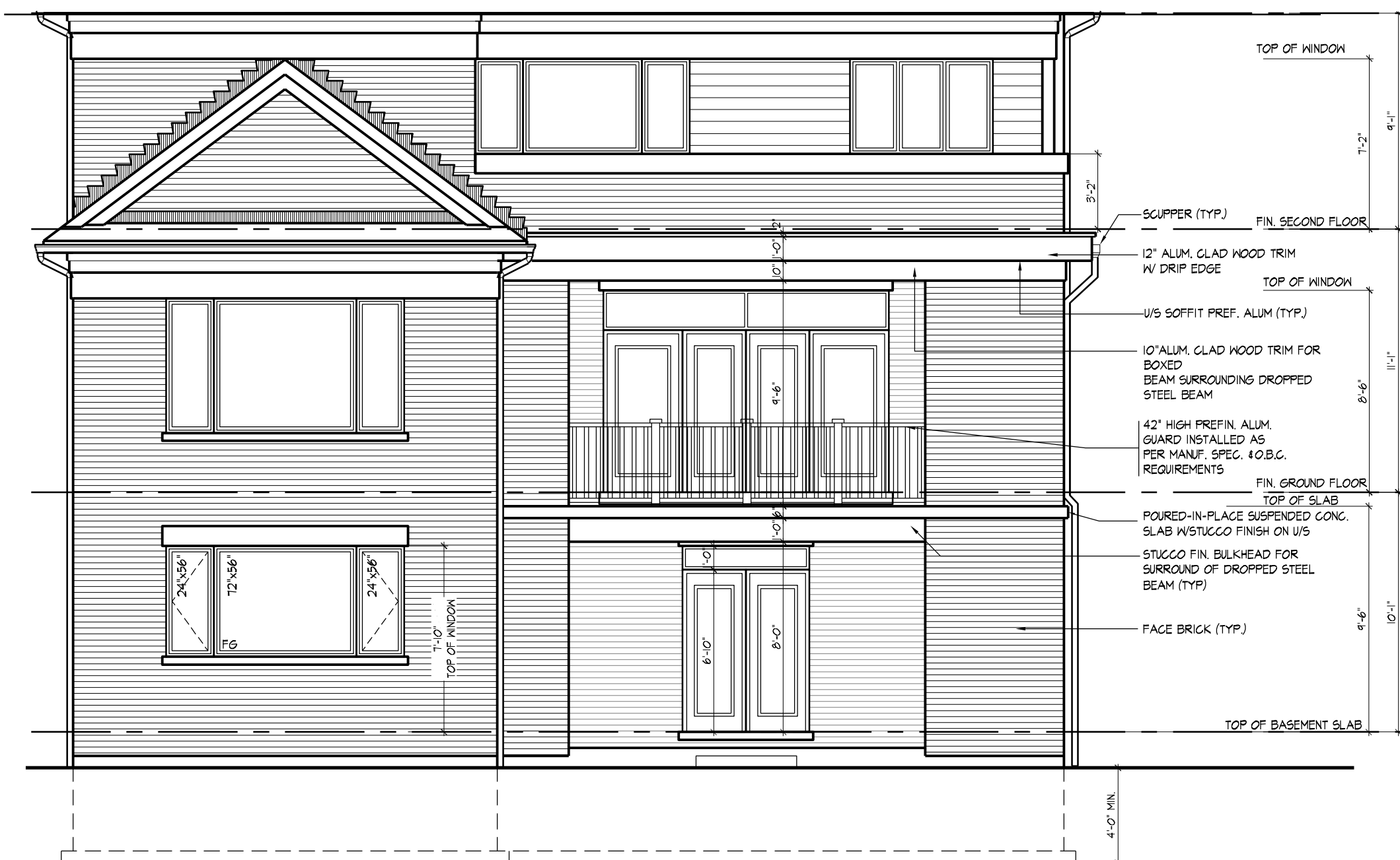
PART. REAR ELEVATION 'C' (LOGGIA/W.O.B. CONDITION)
