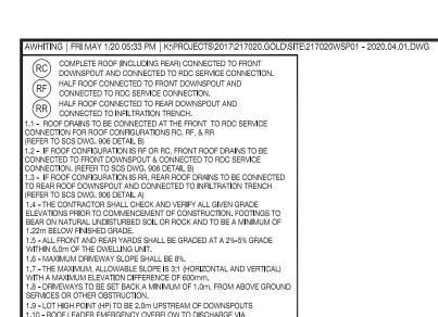
1.10 - ROOF LEADER EMÉRGENCY OVERFLOW TO DISCHARGE VIA SPLASH PAD. (REFER TO SCS DWG. 906 DETAIL A FOR ROOF CONFIGURATION RR AND DETAIL B FOR ROOF CONFIGURATION RC & RF) CONFIGURATION RH AND DETAIL B FOR ROOF CONFIGURATION RC & RF)
