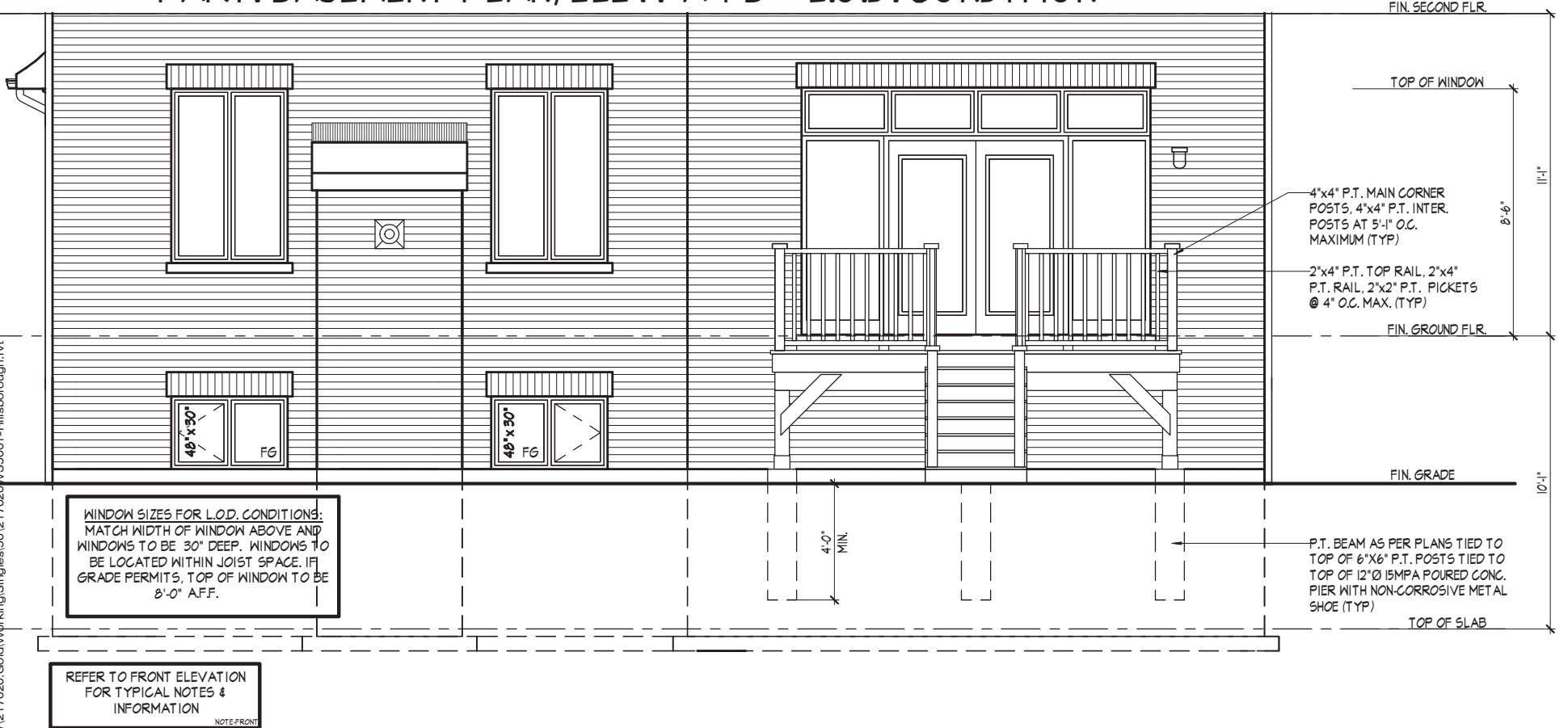
PART. REAR ELEVATION, 'A' & 'B' - L.O.D. CONDITION
