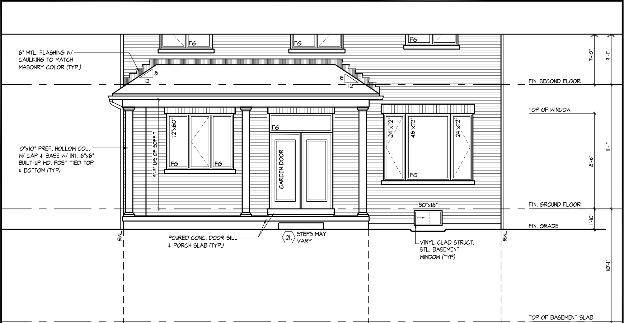
PART. REAR ELEVATION 'A' - OPT. LOGGIA COND. (ELEV. 'B' & 'C' SIMILAR)
