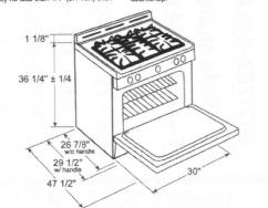
For all installations, install the required rear trim to back of range with 4 screws provided.
