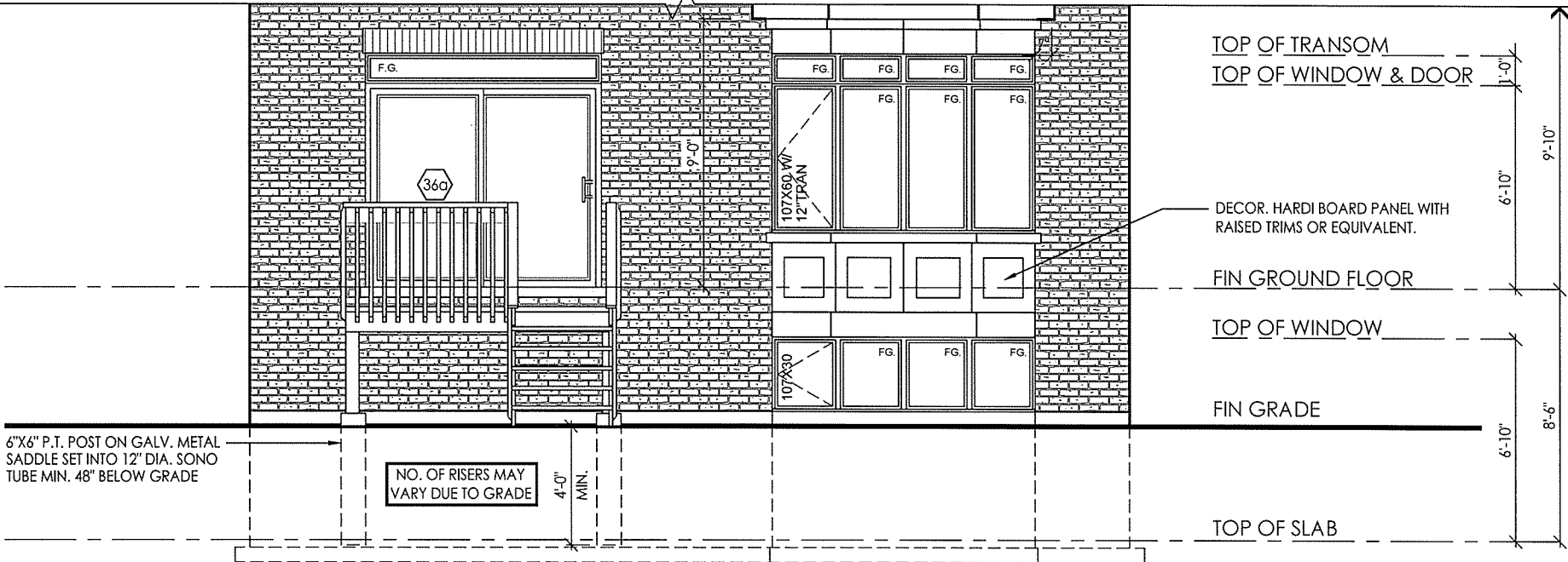
PARTIAL REAR ELEVATION 'A' & 'B' LOB CONDITION
