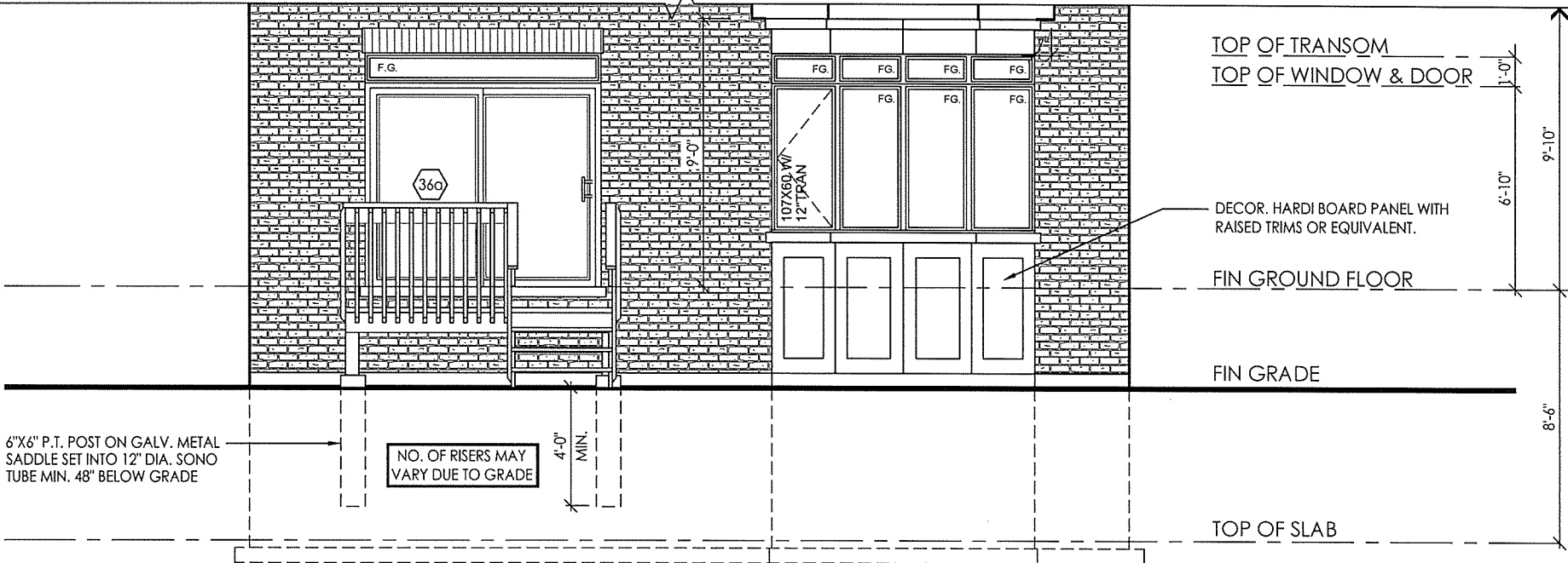
PARTIAL REAR ELEVATION 'A' & 'B' WOD CONDITION
