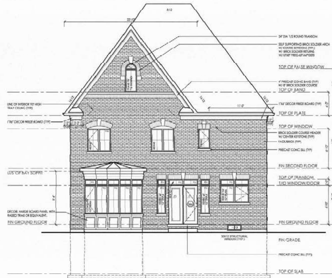
UPGRADED REAR ELEVATION 'A' Lot 3, 7
