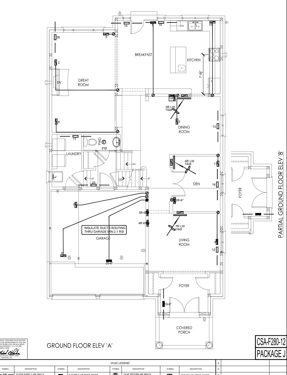
FLOOR SUPPLY AIR GRILLE 14"x8" RETURN AIR GRILLE RETURN AIR STACK ABOVE 6" SUPPLY AIR BOOT ABOVE FLOOR SUPPLY AIR GRILLE 6" BOOT 30"x8" RETURN AIR GRILLE 0 SUPPLY AIR STACK FROM 2nd FLOOR Description Date × RETURN AIR STACK 2nd FLOOR FRA- FLOOR RETURN AIR GRILLE REDUCER SUPPLY AIR BOOT ABOVE **REVISIONS** -6" SUPPLY AIR STACK 2nd FLOOR
