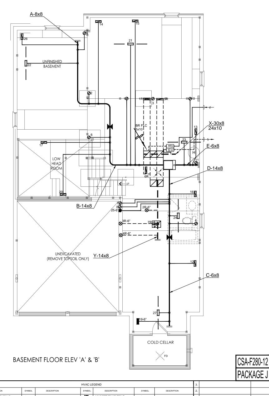
SYMBOL DESCRIPTION 14"x8" RETURN AIR GRILLE FLOOR SUPPLY AIR GRILLE RETURN AIR STACK ABOVE 6" SUPPLY AIR BOOT ABOVE FLOOR SUPPLY AIR GRILLE 6" BOOT 0 30"x8" RETURN AIR GRILLE SUPPLY AIR STACK FROM 2nd FLOOR × Description Date RETURN AIR STACK 2nd FLOOR FRA- FLOOR RETURN AIR GRILLE REDUCER SUPPLY AIR BOOT ABOVE **REVISIONS** -6" SUPPLY AIR STACK 2nd FLOOR
