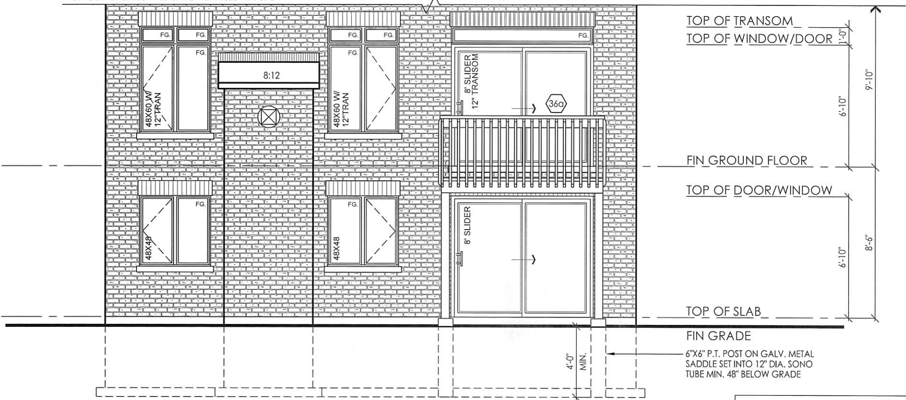
PARTIAL REAR ELEVATION 'A' WOB CONDITION
