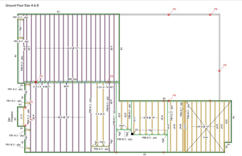
Building Code NBCC 2015 / OBC 2012 Floor Loads Live 40 Dead 15 **Deflection Joist** 360 LL Span L/ 240 TL Span L/ LL Cant 2L/ 720 TL Cant 2L/ 720 Deflection Girder LL Span L/ 360 240 TL Span L/ LL Cant 2L/ 720 TL Cant 2L/ 720 Decking SPF Plywood Deck Thickness Fastener Nailed & Glued Vibration
