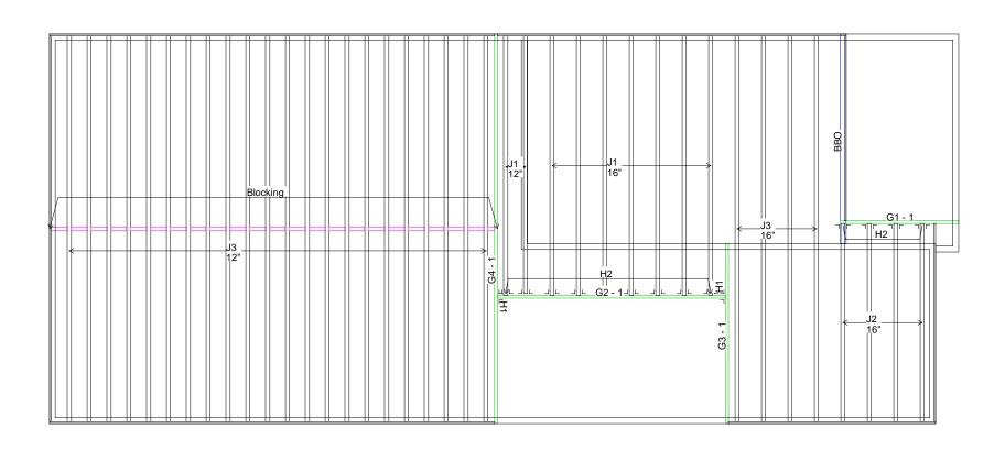
See attached sealed span charts for all uniformly loaded beams. "ALL JOISTS UNDER TILED APPLICATIONS SHALL CONFORM TO OBC 9.30.06"
