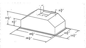
Air Flow Volume: 550 CFM Electrical Connection: 120V/60Hz Electrical Consumption: 200 watts
