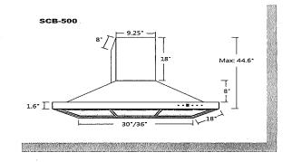
Air Flow Volume: 550 CFM Electrical Connection: 120V/60Hz
