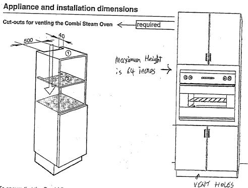
To ensure that the Combi Steam Oven has adequate ventilation, the following cut-outs measuring 19 11/16" x 1 9/16" (500 x 40 mm) must be made:
