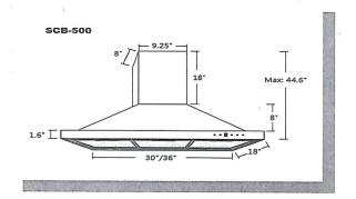
Air Flow Volume: 550 CFM Electrical Connection:
