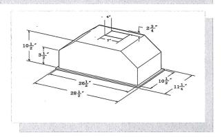
Air Flow Volume: 550 CFM Electrical Connection: 120V/60Hz Electrical Consumption: 200 watts
