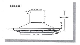
Air Flow Volume: 550 CFM Electrical Connection: Electrical Consumption:
