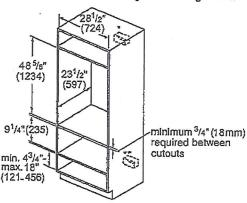
measurements in inches (mm) \*Wall oven junction box may be located above or right or left of the unit within reach of the power conduit. Flush Installation Combination Oven over Storage or Warming Drawer
