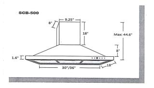
Air Flow Volume: 550 CFM Electrical Connection:
