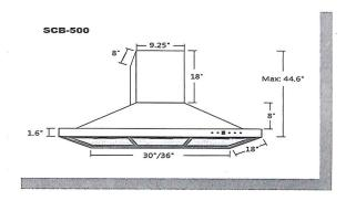
Air Flow Volume: 550 CFM Electrical Connection: 120V/60Hz
