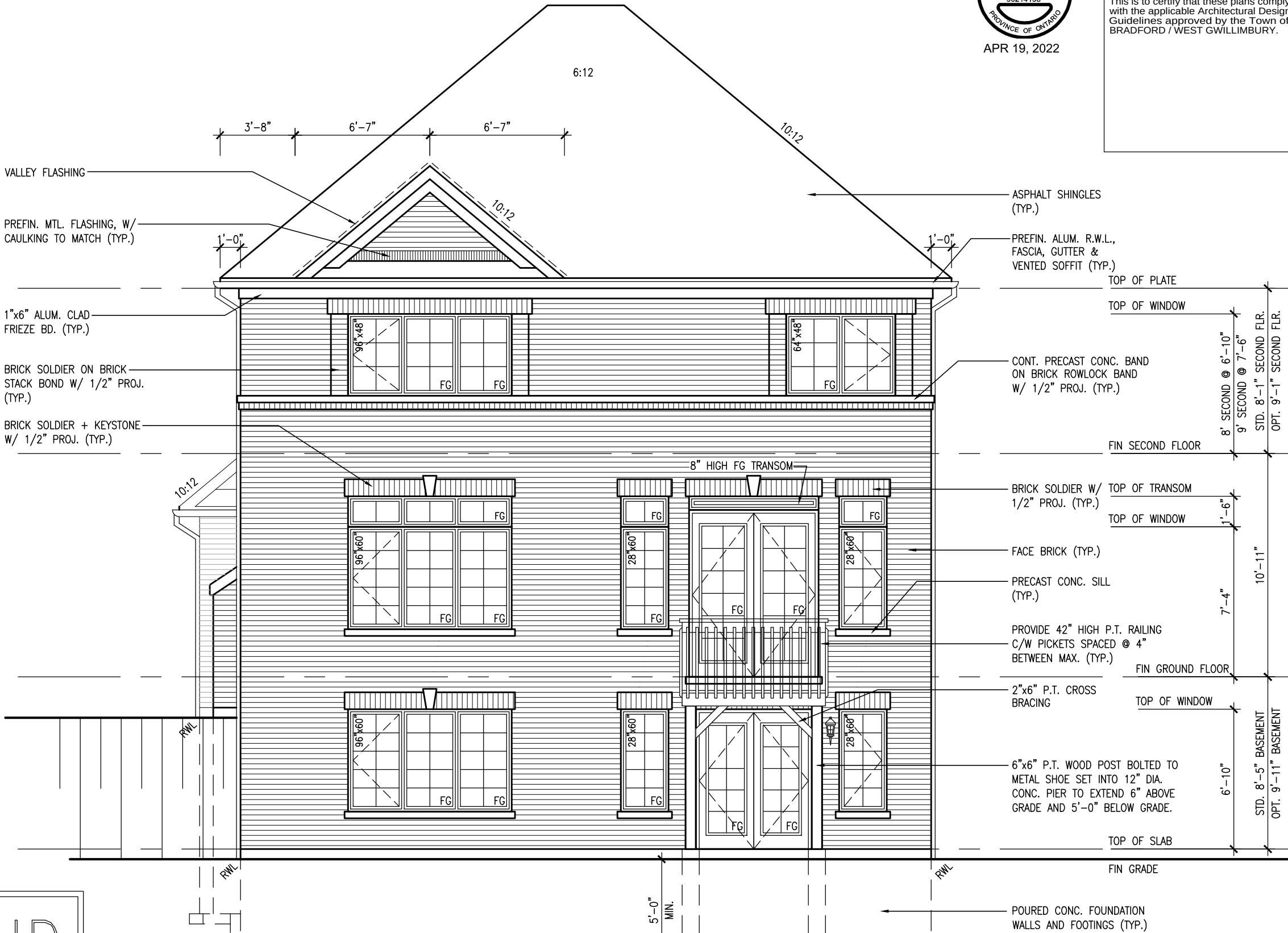
UPGRADED REAR ELEVATION 'A' W/ W.O.B. CONDITION
