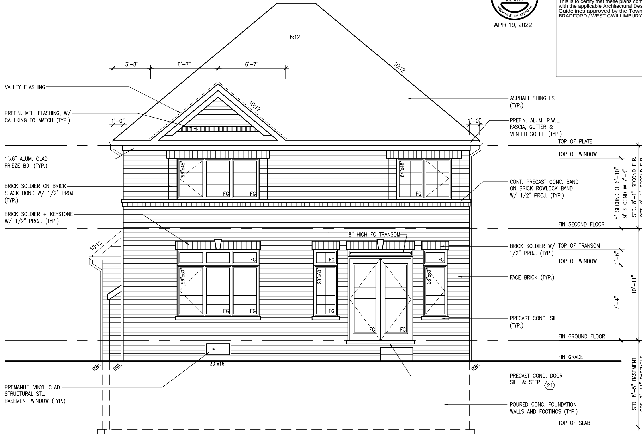
UPGADED REAR ELEVATION 'A'
