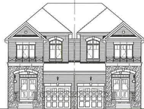
POURED IN PLACE STAIRS WITH MASONRY VENEER LOT # 64R - FRONT ELEVATION SD25-3 -EL. B 12" BRICK DEEP POURED IN PLACE STAIRS WITH MASONRY VENEER ON BOTH SIDES LOT # 64R - FRONT ELEVATION SD25-3 -EL. B (REV.)
