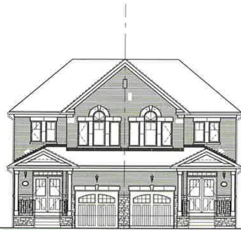
POURED IN PLACE STAIRS WITH MASONRY VENEER ON BOTH SIDES LOT # 70L - FRONT ELEVATION SD25-2 -EL. B
