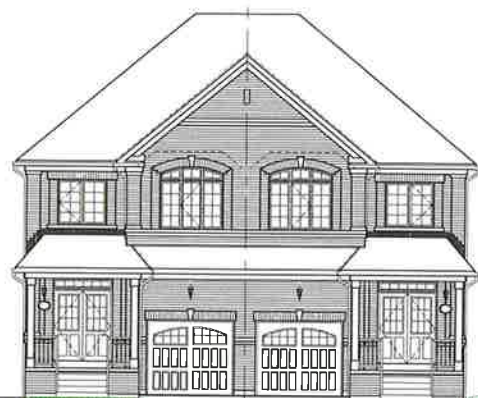
POURED IN PLACE STAIRS WITH MASONRY VENEER ON BOTH SIDES LOT # 65R - FRONT ELEVATION SD25-4 -EL. A POURED IN PLACE STAIRS WITH MASONRY VENEER ON BOTH SIDES LOT # 65R - FRONT ELEVATION SD25-4 -EL. A (REV.)
