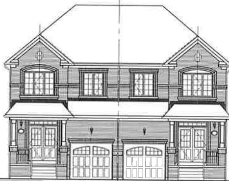
POURED IN PLACE STAIRS WITH MASONRY VENEER ON BOTH SIDES LOT # 71L - FRONT ELEVATION SD25-3 -EL. A
