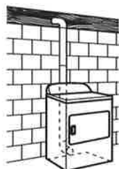
Standard rear offset exhaust installation
