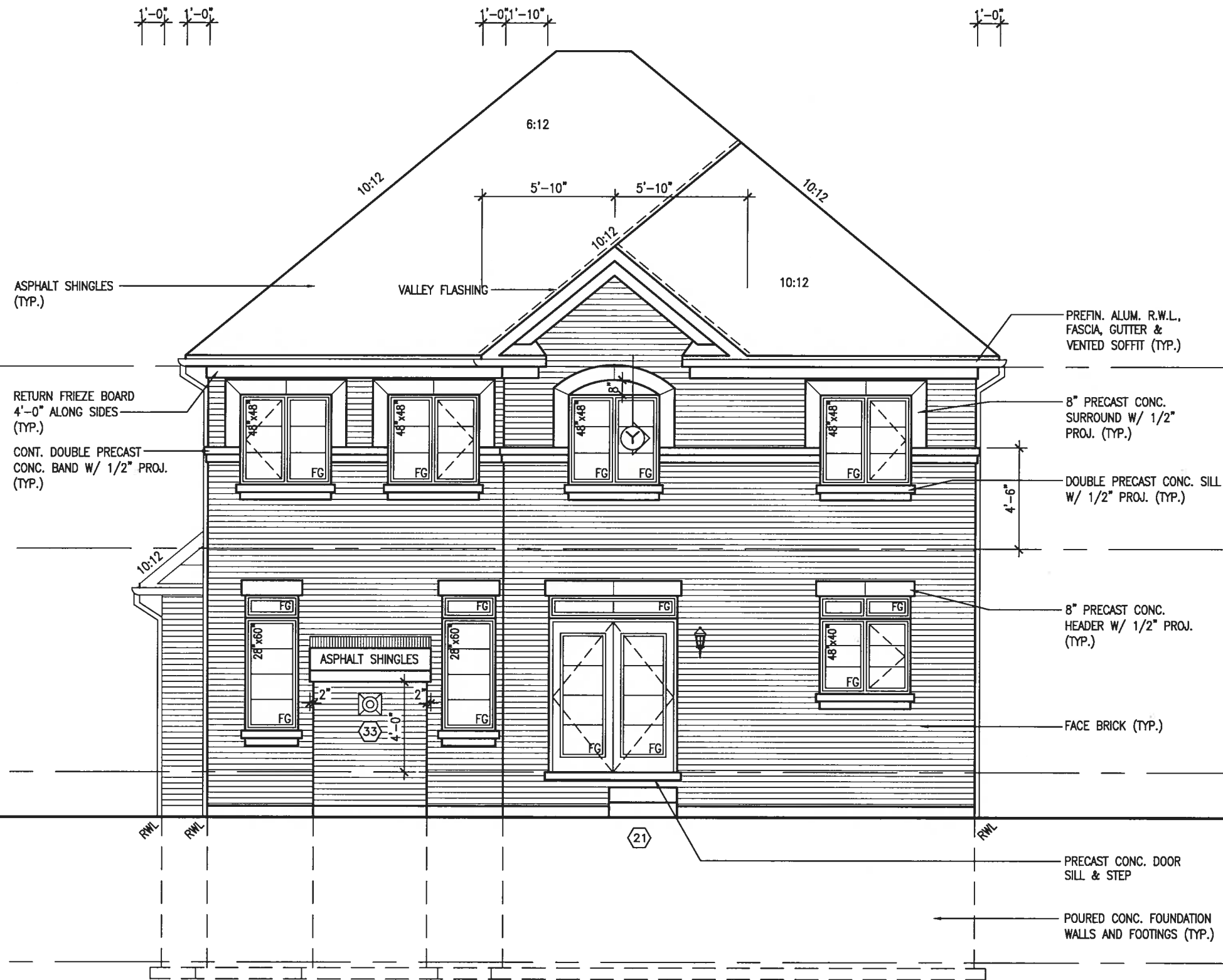
UPGRADED REAR ELEVATION 'B'
