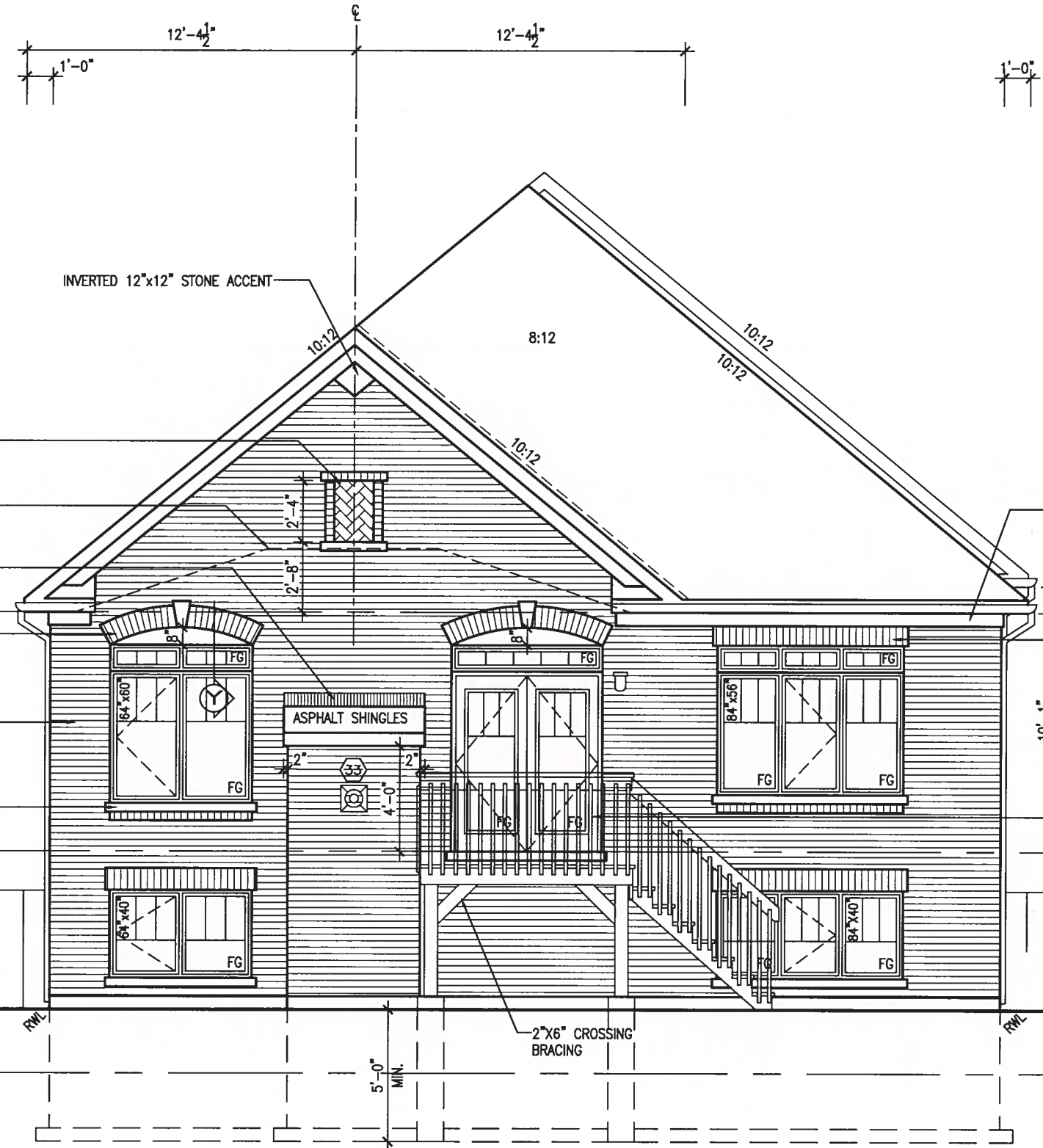
UPGRADED REAR ELEVATION 'A' 9R WOD
