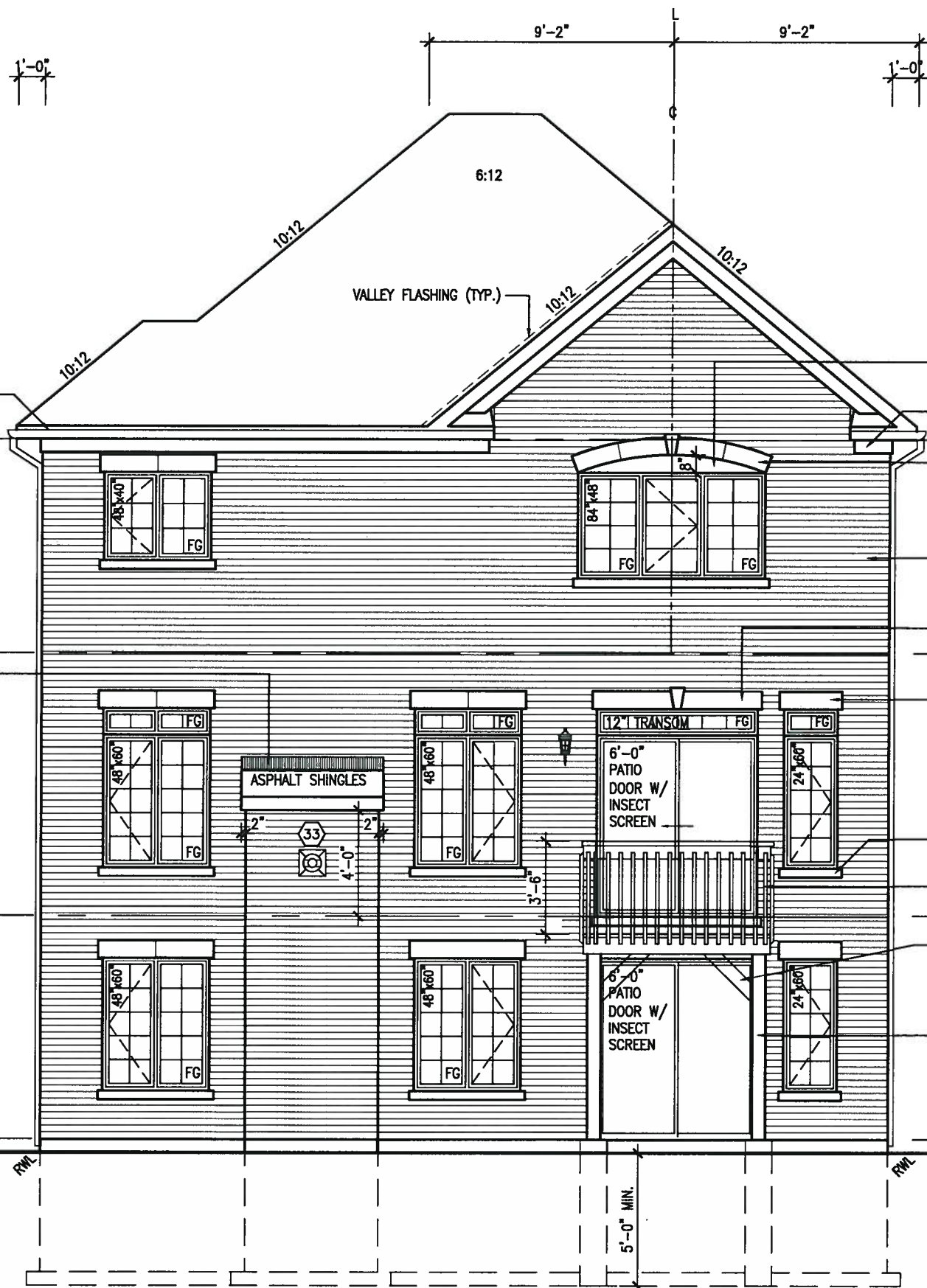
UPGRADED REAR ELEVATION 'B' - W.O.B. CONDITION
