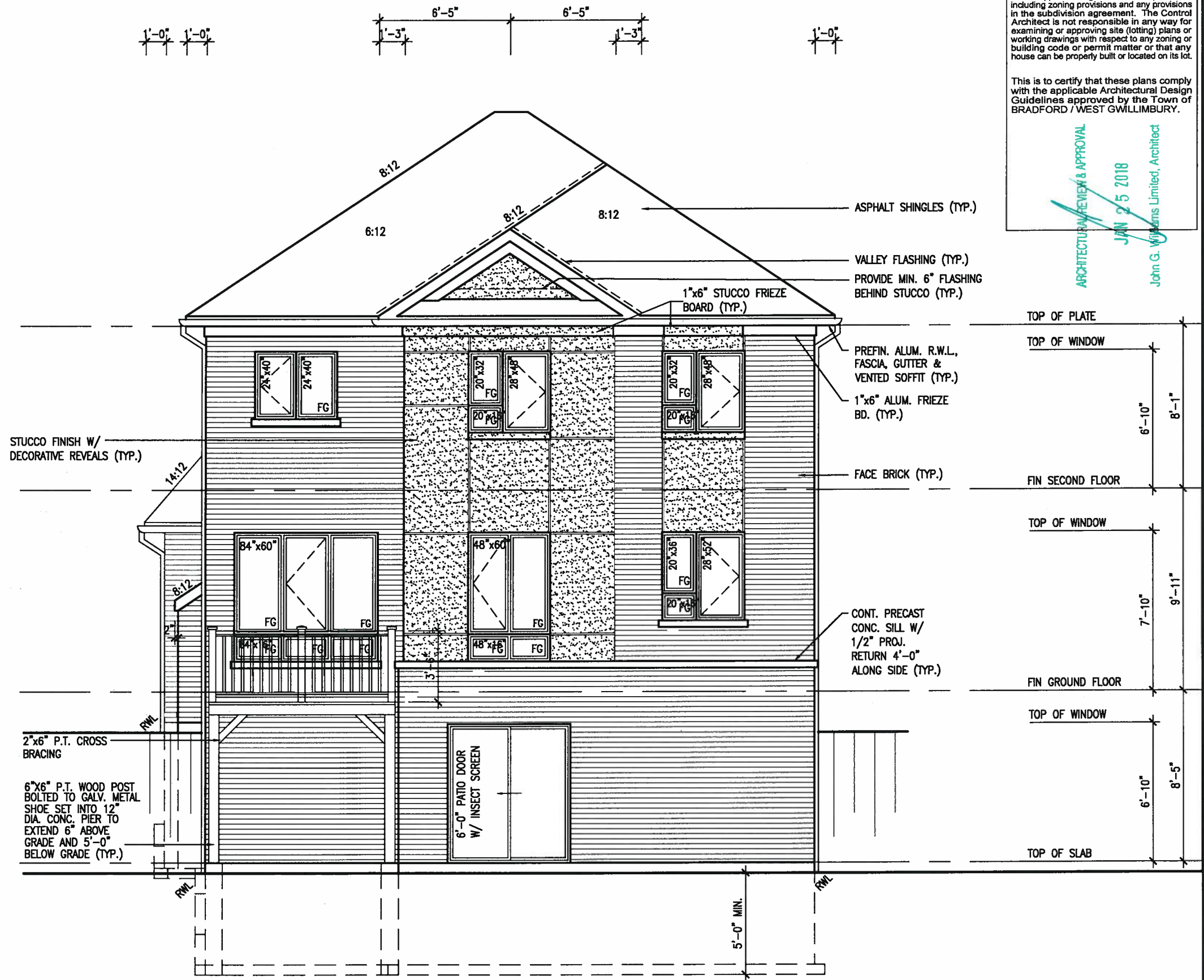
UPGRADED REAR ELEVATION 'C' W.O.B. CONDITION
