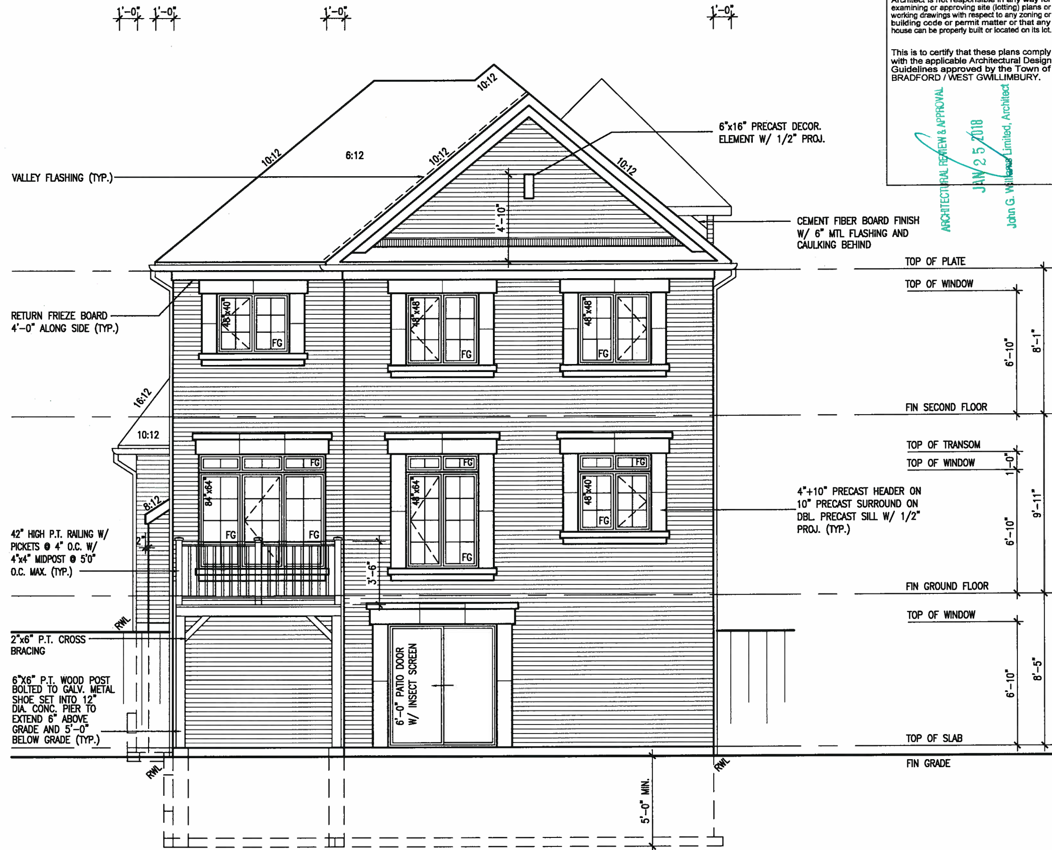
UPGRADED REAR ELEVATION 'B' W.O.B. CONDITION
