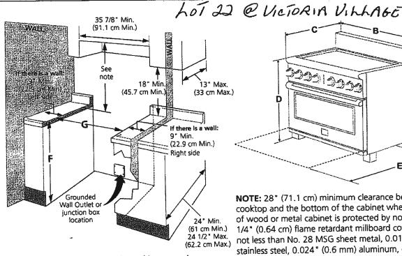
NOTE: 28° (71.1 cm) minimum clearance between the cooktop and the bottom of the cabinet when the botton of wood or metal cabinet is protected by not less than 1/4" (0.64 cm) flame retardant millboard covered with not less than No. 28 MSG sheet metal, 0.015" (0.4 mm) stainless steel, 0.024 ° (0.6 mm) aluminum, or 0.020 ° (0.5 mm) copper.
