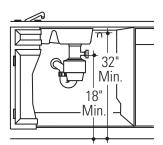
Install waste tee or disposer and air gap according to manufacturer's instructions.
