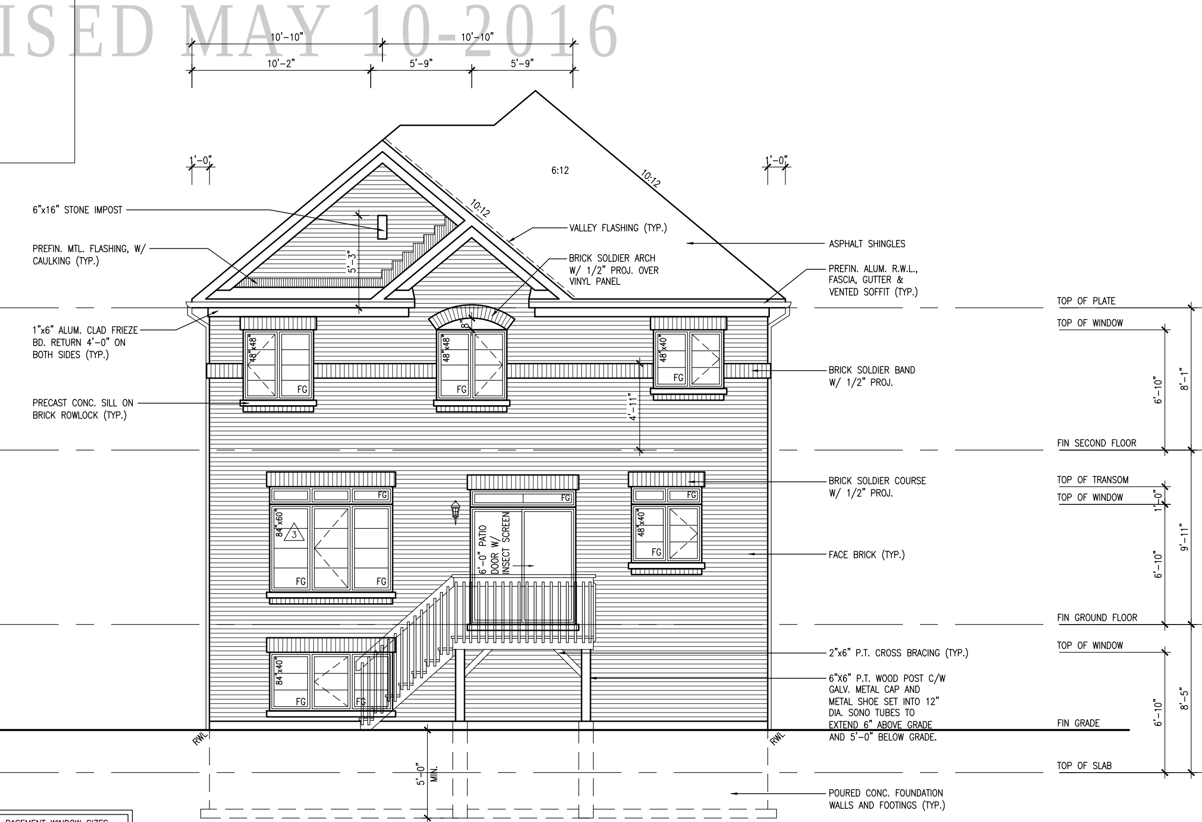
UPGRADED REAR ELEVATION 'B' W.O.D. CONDITION
